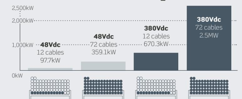
The figure above demonstrates the difference in current-carrying capacity between 48Vdc and 380Vdc configurations. Using the same cable, it can carry 7 times more current than when used to carry 48Vdc. In fact, the 380Vdc stack of 12 cables can deliver 87% more power than the 48Vdc stack of 72 cables.
