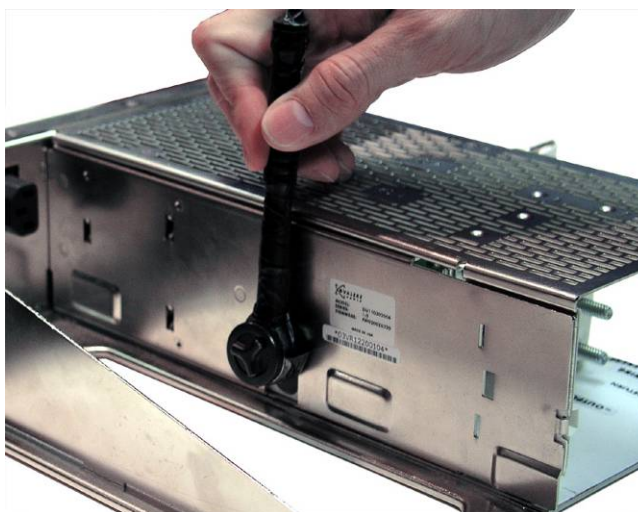
Figure 15 - Removal of the LVD Screw
