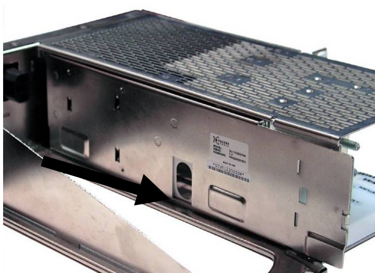
Figure 16 - Removal of the LVD Plate
